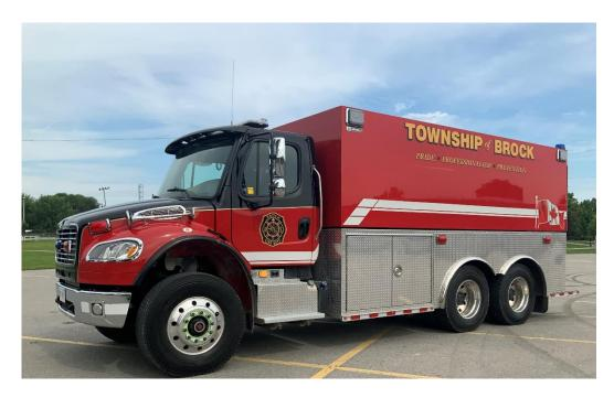
Tank 83 --- 2019 Freightliner commercial cab tanker truck, 3000 US gallons of water, 2<sup>nd</sup> run fire apparatus.
