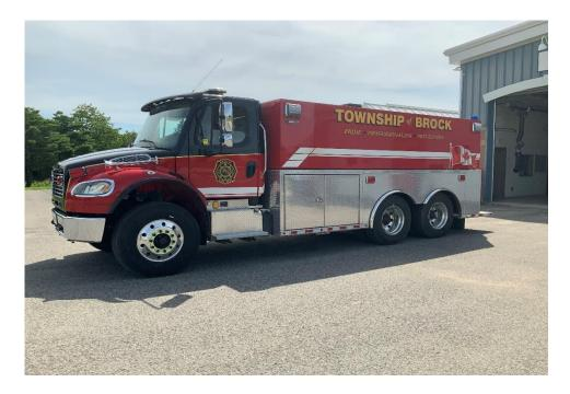
Tank 81 --- 2018 Freightliner commercial cab tanker truck, 2500 US gallons of water, 2<sup>nd</sup> run fire apparatus.
